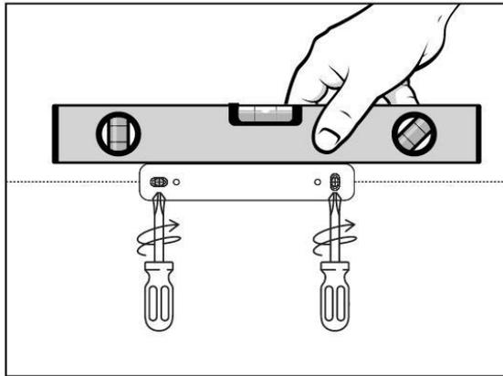
Fit plate using suitable screws. Ensure this is
