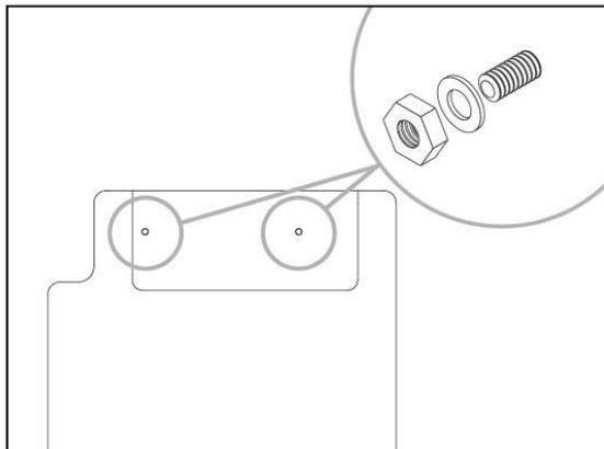
Secure the cistern by placing a washer and nut
